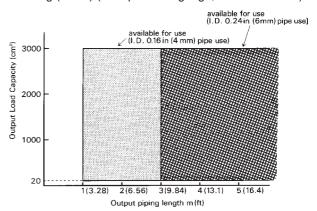
Figure 2. Relationship between Output Load Capacity and Piping Length
